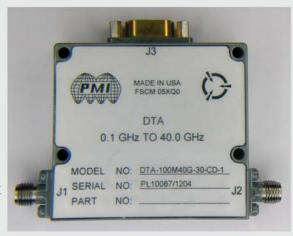
PMI's proprietary digital calibration techniques. This model offers excellent attenuation flatness over the full 100MHz to 40GHz frequency range and operate with input power levels up to +20dBm. This unit is supplied in a very small housing that measures 2.0 x 1.8 x 0.5 inches.
